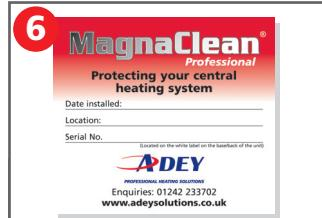
Run the central heating system while checking for leaks. Attach the self-adhesive *MagnaClean* label to the boiler indicating the date of installation, serial number and location of the filter. If necessary, service the filter before leaving the premises. The *MagnaClean Professional* lid spanner and valve spanner can be left with the customer.
